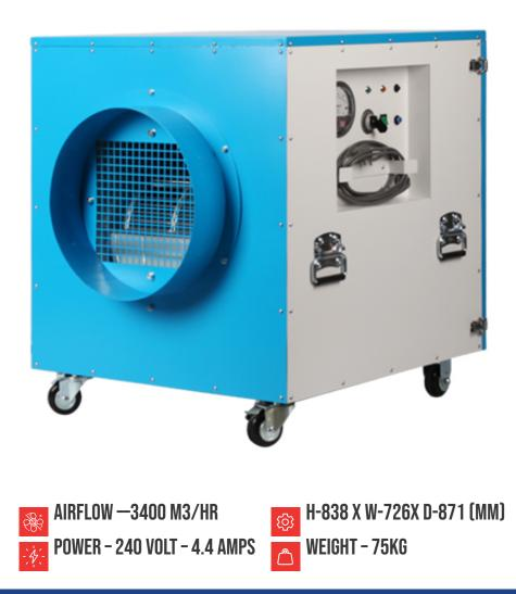
The WAS 3400 Air Filtration Device is a compact portable high performance air purifier. For maximum flexibility it features variable airflow . It delivers 3400 m3/hr of H13 HEPA filtered air while drawing less than 5 amps of power. It features a triple filter to extend filter life and increase purification.
